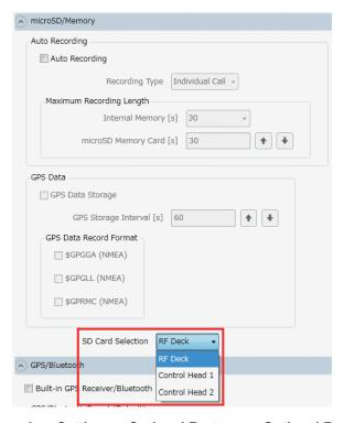
Figure 16-77 KPG-D1 > Transceiver Settings > Optional Features > Optional Features 2 > microSD/Memory If "RF Deck" is configured in SD Card Selection:
