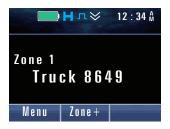
If "%" is used in a string of text when "Unit ID" is configured in **Message Type**, "%" appears replaced with the Unit ID (Own) of the system configured in **Preset System Number**.
