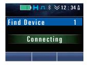
If the selected Bluetooth-compatible device is already registered in the transceiver, the connection process starts by HSP Connection without pairing occurring. Proceed to step 5.
