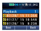
Selecting an audio data folder and pressing the **Menu** ([[]]) key displays the audio data stored in the audio data folder in a list.
