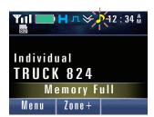
If the audio is recorded to the internal memory, **Auto Recording** does not start if **First-in First-out Deletion** is disabled, and if the maximum number of recordings has already been reached. Also, if the audio is recorded to a microSD card, **Auto Recording** does not start if the conditions for storing data in the microSD card are not satisfied. (Refer to Conditions that enables audio data file and GPS data file to be stored in a microSD card.)
