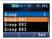
Options for a function, such as "ON" and "OFF", can be selected by pressing the  $[\blacktriangle]$  or  $[\blacktriangledown]$  key and then can be determined by pressing the **Menu** ( $[\Box]$ ) or [\*] key.
