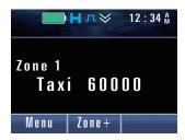
When "Unit ID Name" is configured in **Message Type**, the string of the Unit ID Name (Own) of the system configured in **Preset System Number** appears. If no Unit ID Name (Own) of the system is configured in **Preset System Number**, nothing appears.
