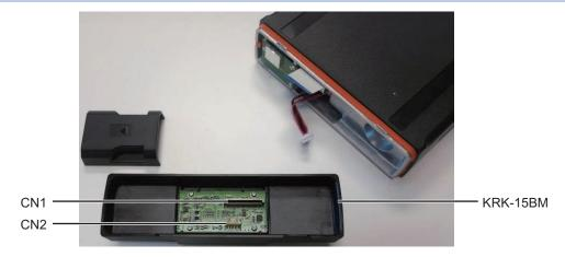
Figure 17-3 Connection of the Cables
