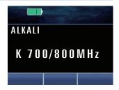
The transceiver enters Panel Test Mode after a lapse of 2 sec.
