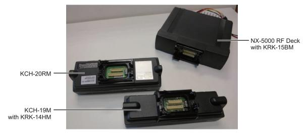
Figure 17-7 NX-5000 RF Deck with KRK-15BM/ KCH-19M with KRK-14HM/ KCH-20RM
