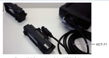
Figure 17-8 Connection of the KCT-71 Cables
