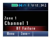
If GPS/Bluetooth Reset is executed in such case, the normal status of the GPS/Bluetooth device is restored and the Bluetooth function can be used.
