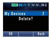
Pressing and holding the key causes the screen to confirm whether to deregister all Bluetooth-compatible devices to appear.
