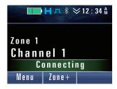
\*If a Bluetooth-compatible device is registered in the transceiver, "Connecting" does not appear.
